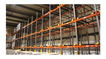
BSE UK also offered good ideas to maximise pallet locations, like adding single pallet racking bays to the end of the cart push back system
